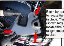
Begin by removing the plastic cover to locate the bolts holding the tail light in place. There should be 3 clips (shown left). Once cover is removed, located the nuts in the back of the tailight housing. Use a wrench or
